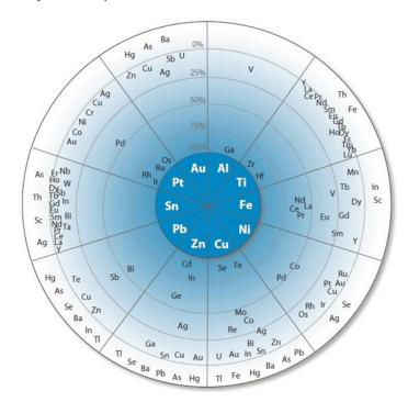
Source: Nassar, Graedel, Harper Sci. Adv. 2015;1:e1400180 3 April 2015 The principal host metals form the inner circle. Companion elements appear in the outer circle at distances proportional to the percentage of their primary production (from 100 to 0%) that originates with the host metal indicated. The companion elements in the white region of the outer circle are elements for which the percentage of their production that originates with the host metal indicated has not been determined.
