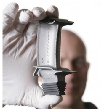
In the last few years, a new wave of superalloys have addressed this issue and include TMS-238, a  $6^{\rm th}$  gen superalloy, which exhibits both high-temperature creep strength and improved oxidation resistance.
